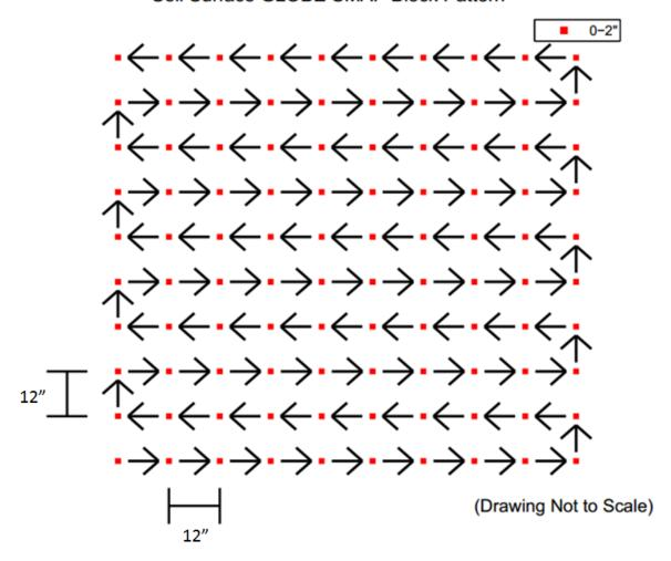
Take all soil moisture measurements one foot (or 30 centimeters) apart continuing in a line for a series of ten samples. On the 11<sup>th</sup> measurement move perpendicular to the previous measurement and continue so on in a snake-like pattern. You may deviate slightly from your sampling site in this idealized model in order to avoid rocks and root clusters. One red dot represents one day of sampling.
